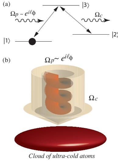
**Figure 1.** (a) The level scheme for the  $\Lambda$ -type atoms interacting with the resonant probe beam  $\Omega_p$  and control beam  $\Omega_c$ . (b) Schematic representation of the experimental set-up with the two light beams incident on the cloud of atoms. The probe field is of the form  $\Omega_p \sim e^{i\ell\phi}$ , where each probe photon carry an orbital angular momentum  $\hbar\ell$  along the propagation axis  $z$ .
