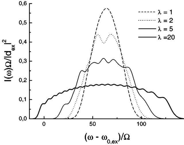
FIG. 1. Absorption line shape calculated using Eq. (6) for  $N = 20$ ,  $T = 0$ , and  $\alpha = 8$ . The singular contributions due to the  $\delta$  functions have been smoothed.
