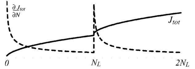
FIG. 2. The current as a function of particle number  $N$  and its derivative clearly show the transition between the Landau levels at  $N=N_L$ .
