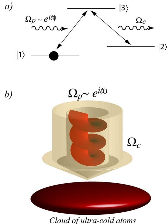
FIG. 1. (Color online) (a) The level scheme for electromagnetically induced transparency with the probe beam and control beams characterized by the Rabi frequencies  $\Omega_p$  and  $\Omega_c$ . (b) The experimental setup with two copropagating light beams and a cloud of cold atoms.
