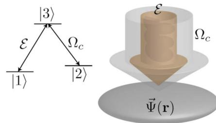
FIG. 1. (Color online) Slow light propagating in a medium of  $\Lambda$ -type atoms.
