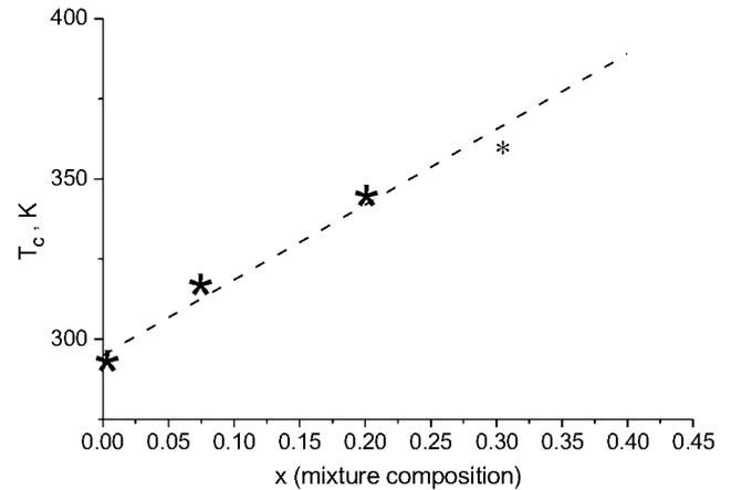
Fig. 3. The dependence of  $T_C$  for  $\text{SbO}_x\text{S}_{1-x}\text{I}$  upon the mixture composition.
