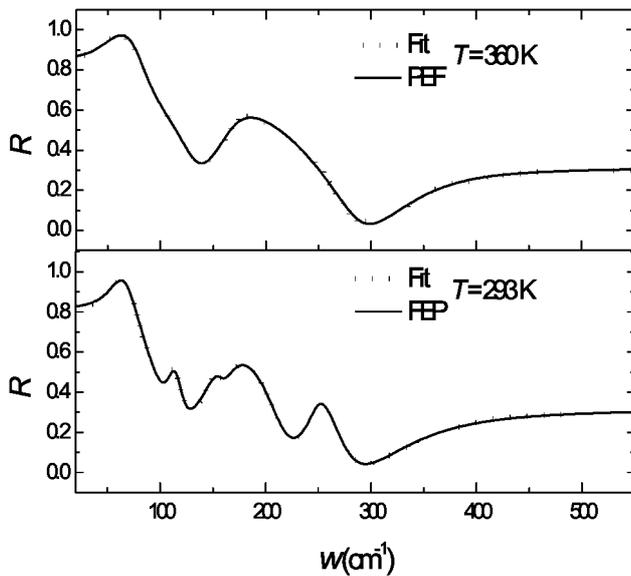
Fig. 4. The reflection spectrum  $R(\omega)$  of the  $\text{SbO}_x\text{S}_{1-x}\text{I}$  ( $x = 0.2$ ) crystals studied by the OP technique at  $\mathbf{E}||\mathbf{c}$  and  $T = 293$  K (FEP),  $T = 360$  K (PEP).
