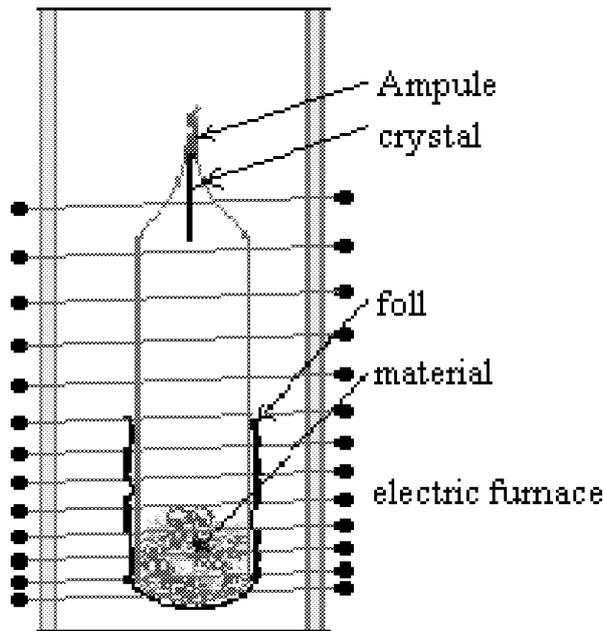
Fig. 1. The furnace for growing the crystals.
