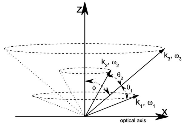
Fig. 1. Schematic depiction of noncollinear phase matching of three plane monochromatic waves in nonlinear crystal.
