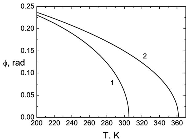
Fig. 2. Dependence of the direction of collinear degenerate parametric interaction (angle  $\phi$ ) on crystal temperature for LiNbO<sub>3</sub> (1,  $\lambda_3 = 0.532 \mu\text{m}$ ) and KDP (2,  $\lambda_3 = 0.266 \mu\text{m}$ ) crystals.
