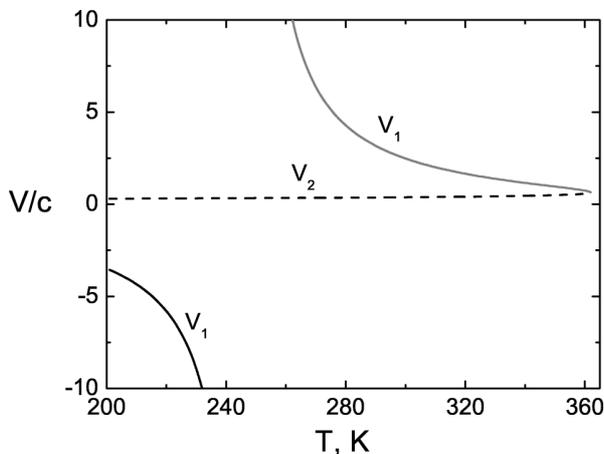
Fig. 4. Dependences of the velocities of two X wave modes on temperature in KDP crystal.  $\lambda_3 = 0.266 \mu\text{m}$ .
