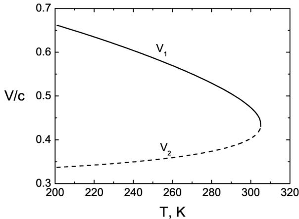
Fig. 3. Dependences of the velocities of two X wave modes on temperature in LiNbO<sub>3</sub> crystal.  $\lambda_3 = 0.532 \mu\text{m}$ .
